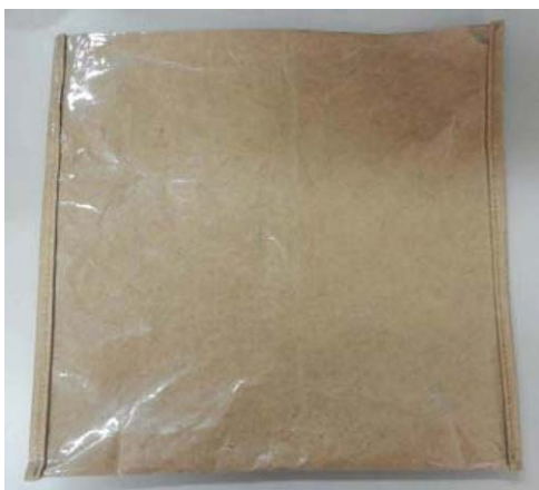
Figure 1. Photo of jute nonwoven/selective barrier film composite bag. [Color figure can be viewed in the online issue, which is available at wileyonlinelibrary.com .]
