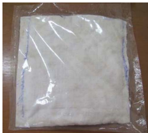
Figure 2. Photo of SAF nonwoven bag covered with selective barrier film. [Color figure can be viewed in the online issue, which is available at wileyonlinelibrary.com .]
